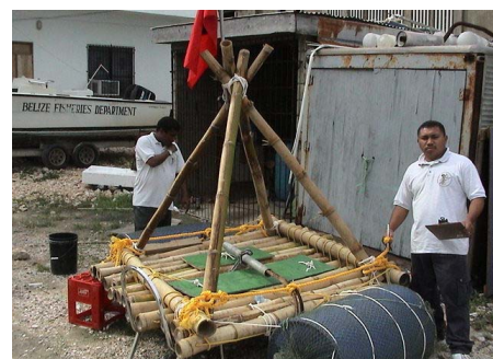
Experimental FAD built from bamboo in Belize
