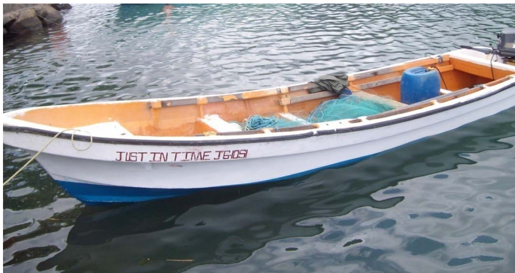
Fibre-glass reinforced Pirogue
