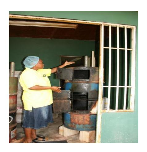
Smoking chamber where the bonito is placed for three hours per batch.
