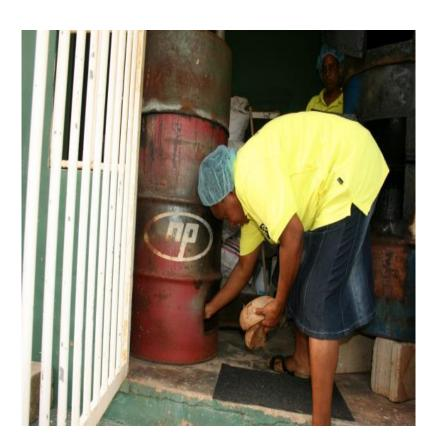
Stacking the smoking chamber with coconut husk. N.B the appropriate technology used for the smoking chamber – an np oil drum.
