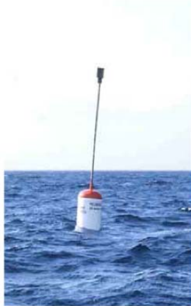
MKII-GRP7 Medium strength current 560 m mooring depth
