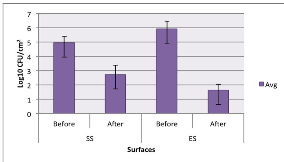
Figure 11: The average total viable count on stainless steel and electropolished stainless steel surfaces from the LL protocol
