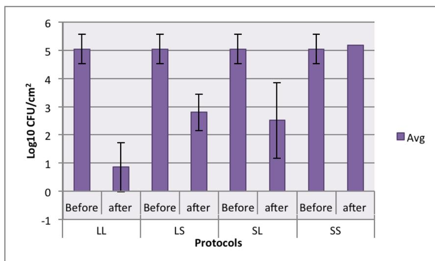
Figure 9: The average total viable count on electropolished stainless steel surfaces
