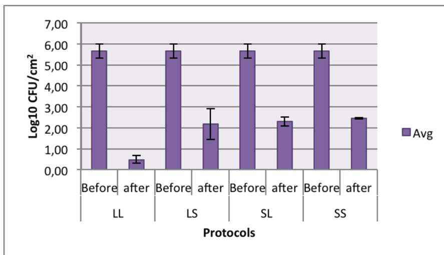
Figure 8: The average total viable count on stainless steel surfaces
