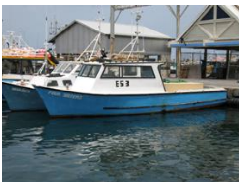
Ice Boat (Wood with detachable ice box)
