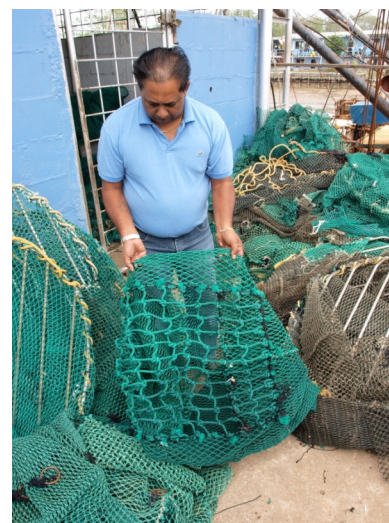
Trawling nets with bycatch reduction device
